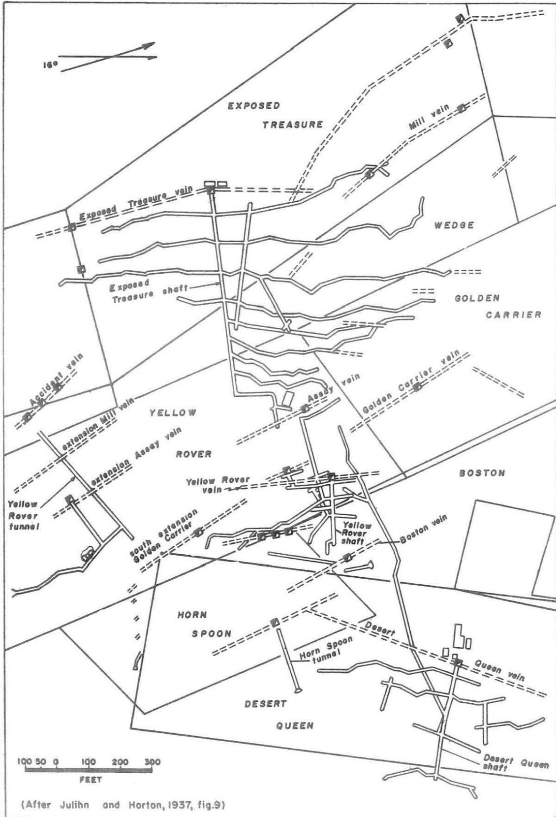
Figure 56. Composite plan of the Standard group (Desert Queen, Exposed Treasure, and Yellow Rover mines).
