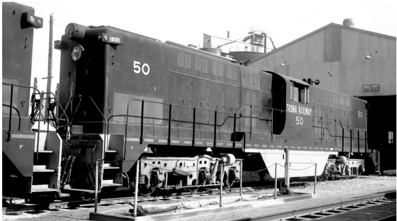
Caption. Both of Trona Railway's rare DT-6-6-2000's can be seen here, acquired from Baldwin as new equipment in 1949. From https://www.american-rails.com/trona.html accessed Nov. 15, 2023.
